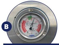
If the pressure is higher than 10 bar, the pump cannot fill the tank.
