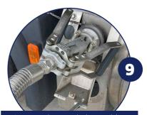
Connect the nozzle by pushing the two LNG handles forwards simultaneously.
