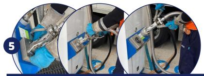
Unlock the LNG nozzle by pulling on the two handles simultaneously, then rotate it by one quarter of a turn to release the nozzle from the stops and detach it.
