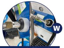
To resume the filling cycle, disconnect the nozzle from the tank, put it back on its support on the pump and rotate by one quarter of a turn to lock it.
