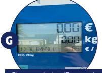
The pump displays "Disconnect downwards" to inform you that the depressurisation cycle has been completed.
