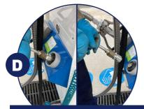
Rotate the vent nozzle by one quarter of a turn to unlock and remove it from its support on the pump.
