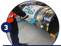
Dry and clean the two tank fittings on the vehicle (LNG and vent) using a compressed air blower or a cloth.
