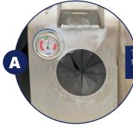
To depressurise the tank, you must monitor the pressure reading on the pressure gauge of the vehicle's tank.
