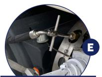
Connect the vent nozzle to the vehicle and rotate by one quarter of a turn to lock it.
