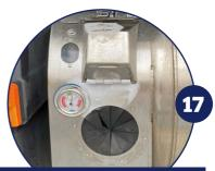
Remove the earthing clamp and close the grey vent valve of the tank.
