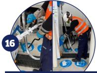
Put the gun back on its support. Position it opposite the stops, turn through 1/4 of a turn and lock by pushing the two handles forwards at the same time.
