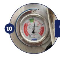
For vehicles other than Volvos, if the pressure in the tank is higher than 10 bar, follow the instructions for depressurisation on page 8.
