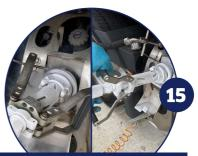
Disconnect the nozzle by pulling the two handles backwards simultaneously. Wait for 3 seconds, then rotate the nozzle by one quarter of a turn to disconnect it from the vehicle.
