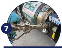
Position the filler nozzle in front of the vehicle filler, aligned with the stops.
