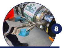
Insert the nozzle in the tank and rotate by one quarter of a turn to lock.
