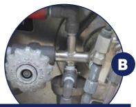
Open the grey vent valves on each of the vehicle's tanks.
