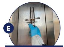
To resume filling, follow the instructions shown on the screen, disconnect the vent nozzle and put it back on its support.
