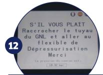
If the pressure in the vehicle's tank is high, follow the instructions for depressurisation.
