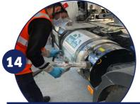
Disconnect the nozzle by pulling the handles backwards. Wait for 3 seconds, then rotate the nozzle by one quarter of a turn to disconnect it from the vehicle.
