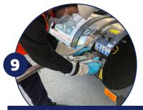
Connect the nozzle by pushing the two LNG handles forwards.
