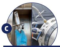
Detach the vent nozzle from its support on the pump and connect it to the vehicle's tank.
