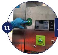
Whenever the visual and sound signals are given, press the "DEAD MAN" button on the pump to prove that you are present and paying attention.
