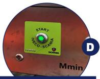
For IVECO SCANIA vehicles, press the "START" (or depressurisation) button to start.
