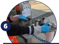
Dry and clean the filler nozzle with compressed air or a cloth.
