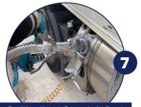
Position the LNG nozzle in front of the vehicle filler, aligned with the stops.
