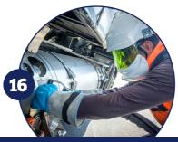
Disconnect the nozzle by pulling back the two handles simultaneously. Wait for 3 seconds, then rotate the nozzle by one quarter of a turn to disconnect it from the vehicle.
