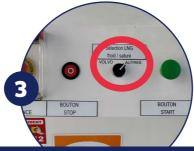
Select the filling mode according to the make of vehicle via the switch on the Dispenser: "VOLVO/AUTRES" (VOLVO/OTHER).
