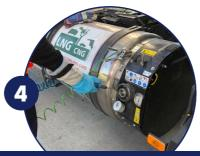
Dry and clean the two tank fittings on the vehicle (LNG and vent) using a compressed air blower or a cloth.
