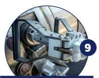
Connect the LNG nozzle by pushing the two handles forwards.
