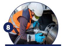
Insert the nozzle in the tank and rotate by one quarter of a turn to lock.
