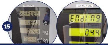
Wait until the screen displays "ENDING" before detaching the nozzle.
