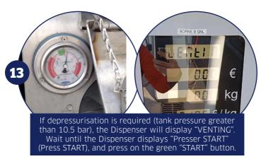
**Note:** The "VENTING" operation ends once the pressure reaches the green zone of the tank's pressure gauge.
