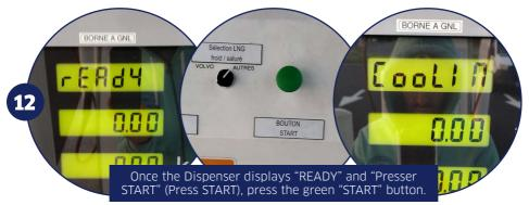
**Note:** After pressing "START", the Dispenser displays "COOLING" and a countdown is begins. The cooling period is automatically established and varies according to the pump's temperature setting.
