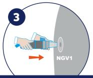
Insert the end of the nozzle in the vehicle's filler inlet and push slightly
