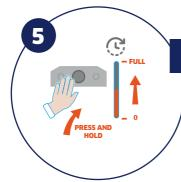
Press and hold the "DEAD MAN" button on the pump until the tank is full
