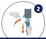
Press the lever to remove the nozzle from its support
