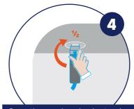
Open the nozzle valve by turning the blue handle by one half turn towards the vehicle
