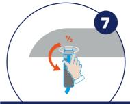
Close the nozzle valve by turning the blue handle by one half turn. Wait 3 seconds for the nozzle to decompress
