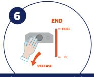
The pump stops automatically when the tank is full.
